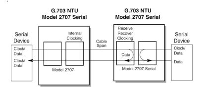
Figure 7. Local Loopback for a Network Termination Application
